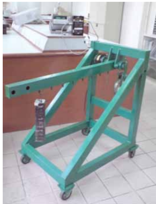
Plate 5. Power measuring instrument, torque and force transducers at the calibration stand
