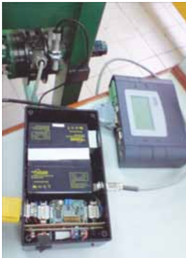
Plate 2. Physical setup of the portable power measuring instrument
